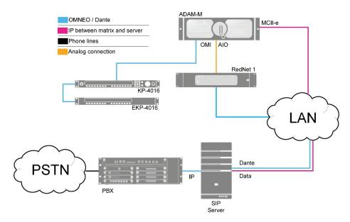
Figure 2. SIP-example using an analog output from the matrix
