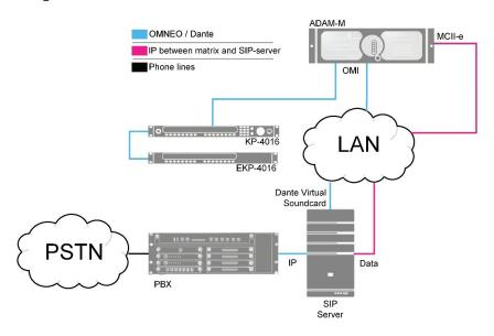
Figure 1. The basic SIP-solution
