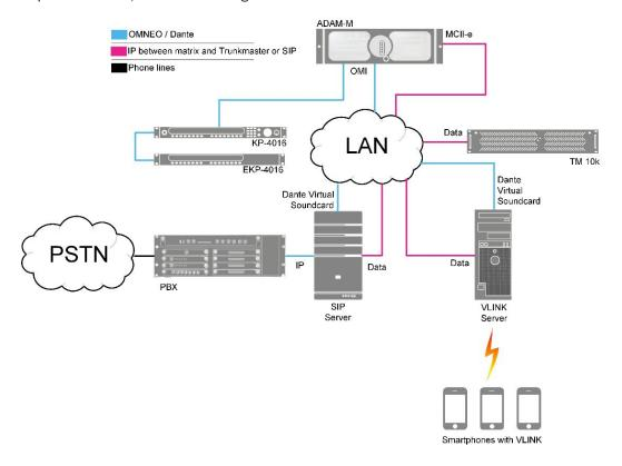
Figure 3. Use of VLINK for SIP and for Smartphones requires two servers
