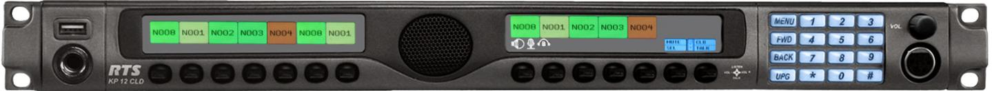
The KP 12 CLD intuitive graphic interface is housed inside two (2) full-color 4.2" LCD displays. The front panel also features conveniences such as a user-programmable buttons, one-touch listen volume adjustment on each of the 14 multifunction keys, and a backlit keypad. Like all RTS products, the KP 12 CLD is designed with expansion in mind. The front-mounted USB port and modular rear panel allow for future upgrades that will keep the KP 12 CLD on the forefront of technology for years to come.
