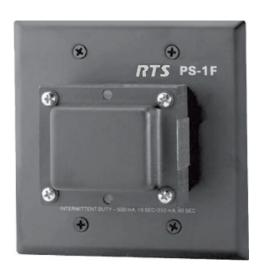
The RTS Audiocom Model PS-1F Power Supply mounts in a standard two-gang electrical outlet box. It may be used to power a single intercom channel containing up to 4 beltpack headset stations.
