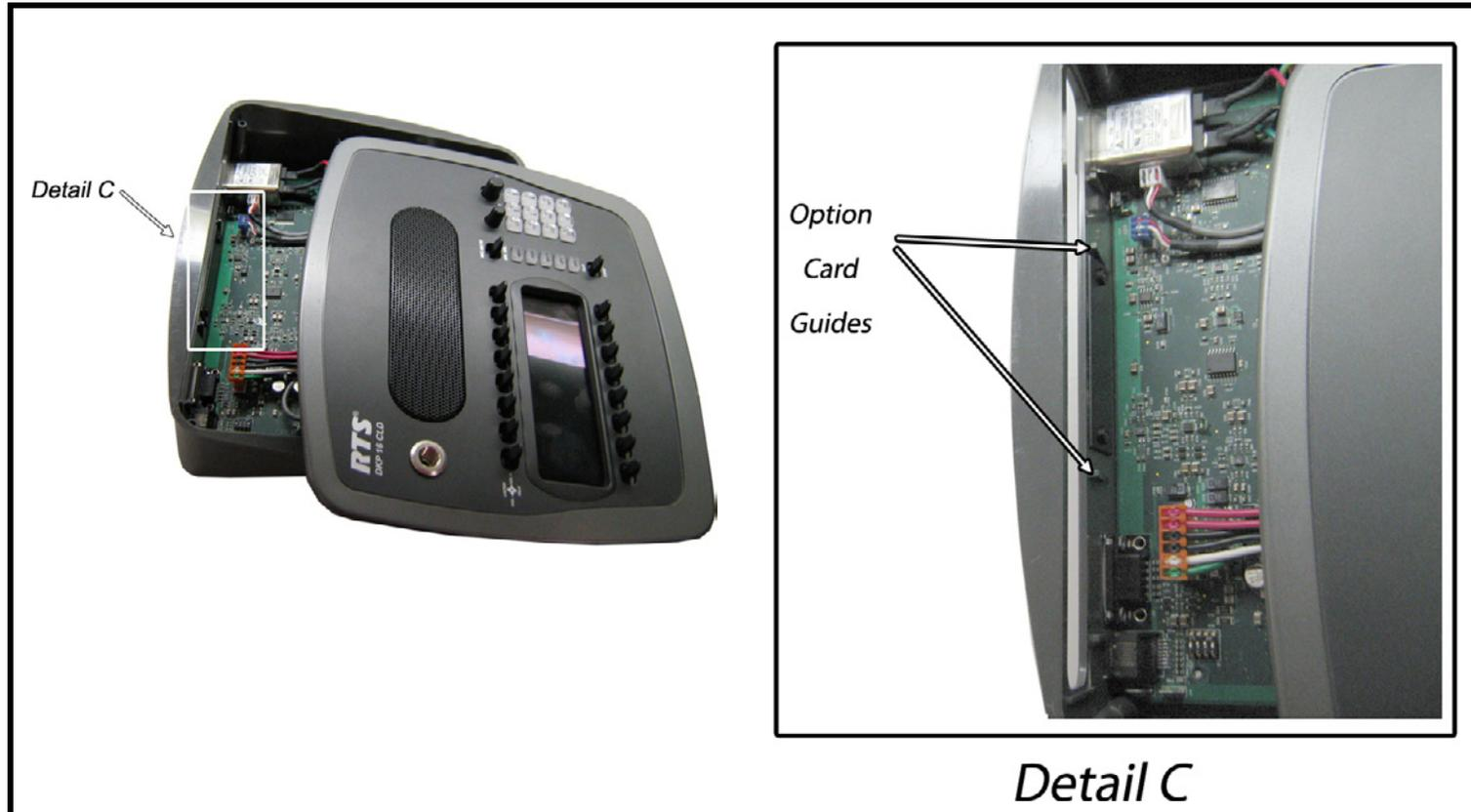
FIGURE 5. GPIO Option Card Guides
