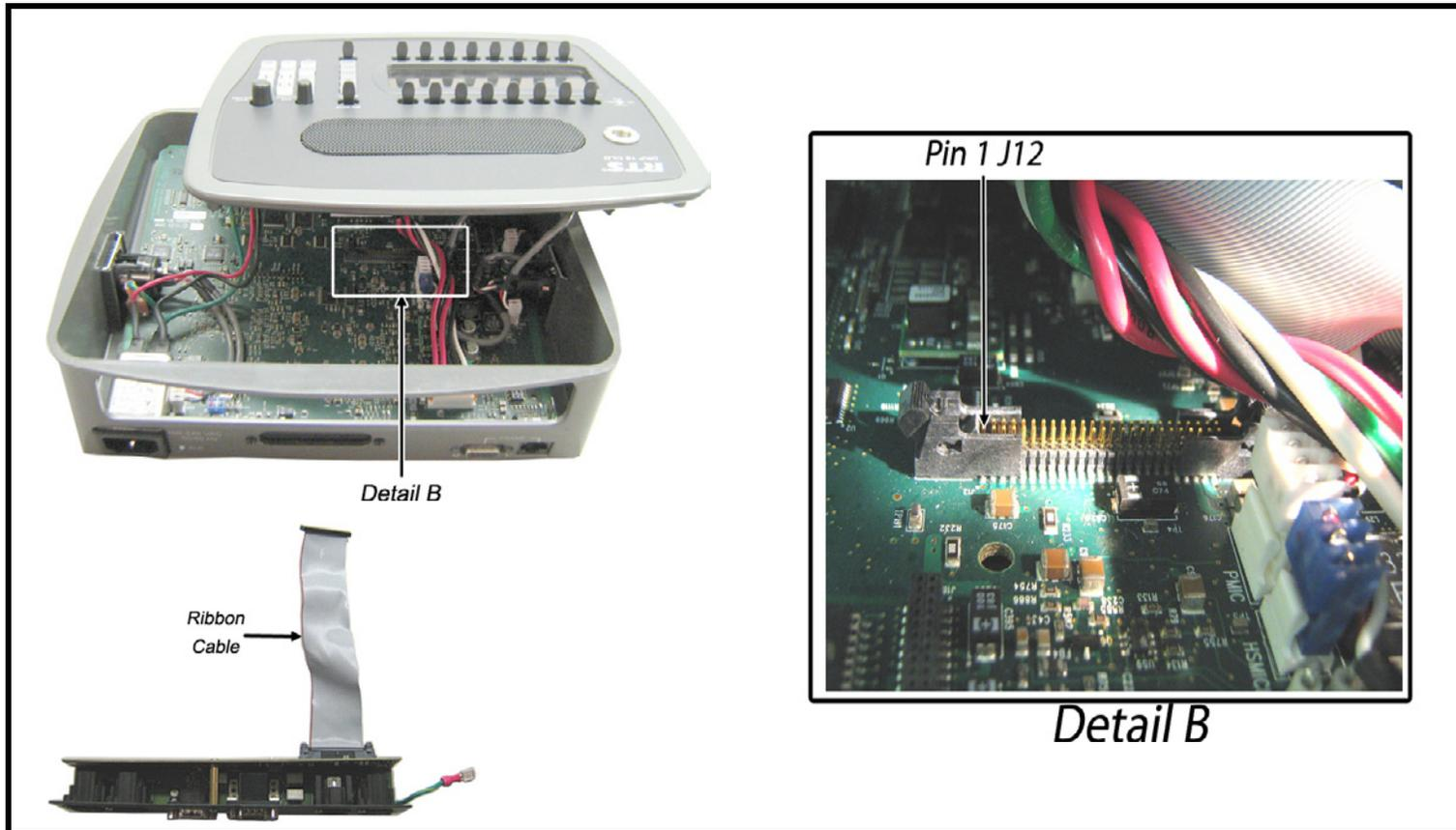
FIGURE 4. Attach the GPIO option card ribbon cable
