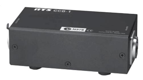
The CCB-1 interfaces a single RTS Audiocom balanced intercom channel to a single Clear-Com unbalanced intercom channel, with full audio and light signaling compatibility between the two (2) intercom channels. The CCB-1 has no controls and is completely transparent to intercom system operation.
