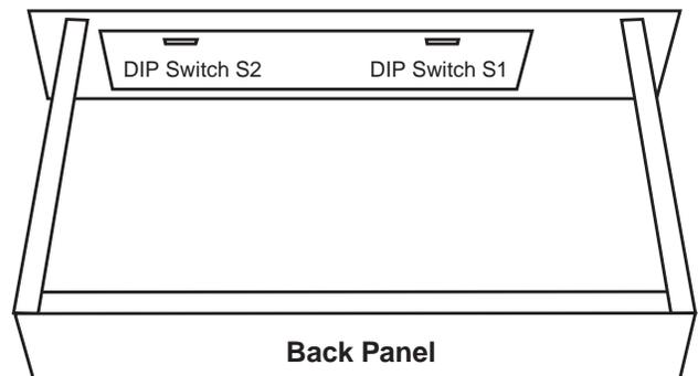
**Figure 4.** *Locations of DIP switches*
