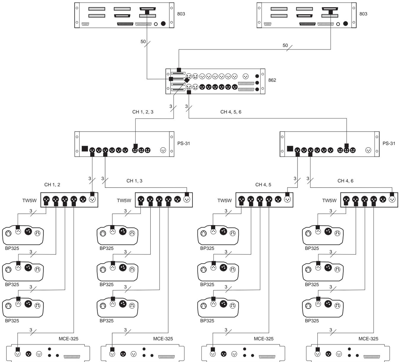
**Figure 16.** An application showing 803 master stations connected to a TW intercom system using an 862 interconnect panel. In this application, each PS-31 provides power to three intercom channels. All intercom stations connected to each power supply can intercommunicate on a common conference channel (channel 1 or channel 4). This channel is not available to the 803's. Each 803, however can selectively communicate with any of the 4 intercom branches on a private channel.
