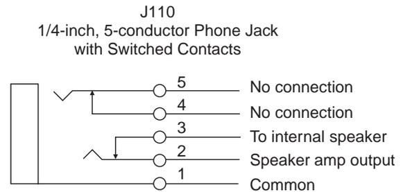
**Figure 9.** J110 connector pin-out
