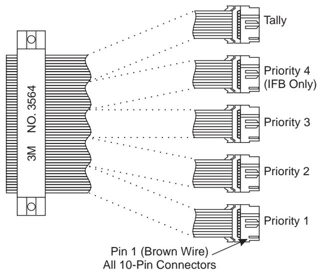
**Figure 2.** Priority and tally connectors for IFB and ISO option cables
