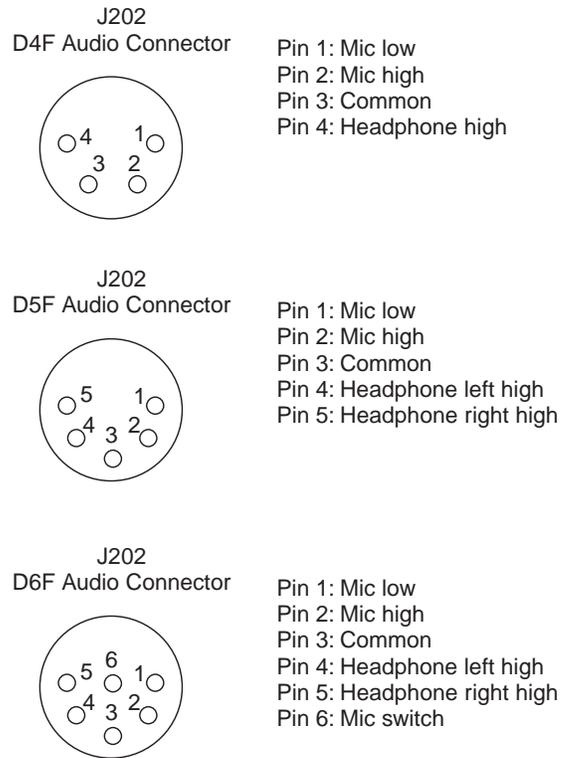
Figure 12. J202 connector pin-outs
