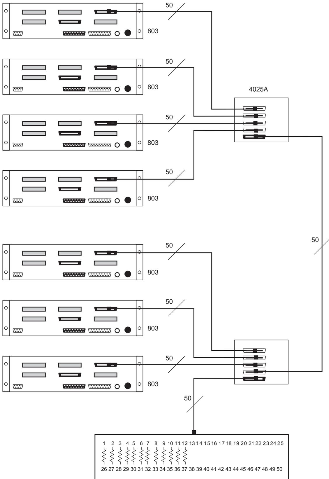
**Figure 17.** A balanced, 2-wire intercom system using only 803 intercom stations. Each intercom station can talk and listen to any one or combination of intercom stations. A 200-ohm resistor is connected across each 2-wire channel to set the terminating impedance. By adding another 4025A interconnect panel, the system could be expanded to 12 stations.
