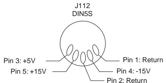
**Figure 10.** J112 connector pin-out (looking toward the back panel)
