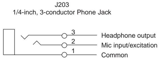
Figure 13. J203 connector pin-out
