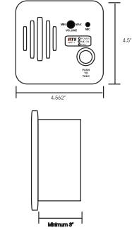
Figure 2. WKP-1 Industrial Keypanel size requirements.
