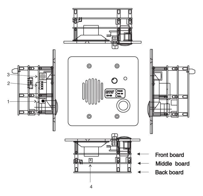
Figure 5. WKP-1 3-dimensional view component boards.
