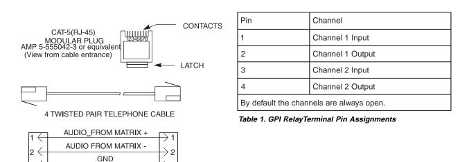
Figure 8. CAT-5 (RJ-45) Intercom cable wiring diagram.
