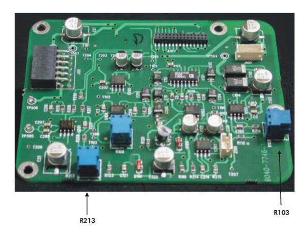
Figure 4. The middle board in the WKP-1 (also referred to as the audio board).
