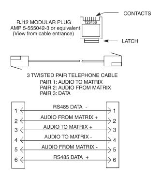
Figure 7. RJ-12 Intercom cable wiring diagram
