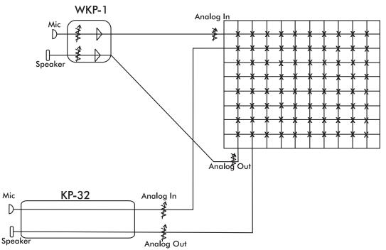
Figure 3. System Diagram depicting Gain Control.
