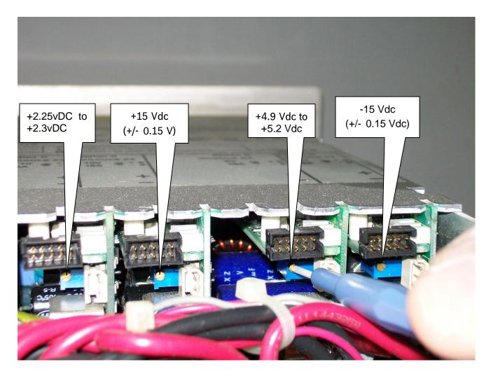
Power up the right side power supply. Power down the left side power supply. Repeat the module voltage measurement and adjustment (if necessary).
