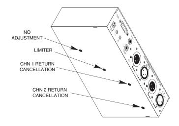
Figure 3. Adjustments Accessible From the Underside
