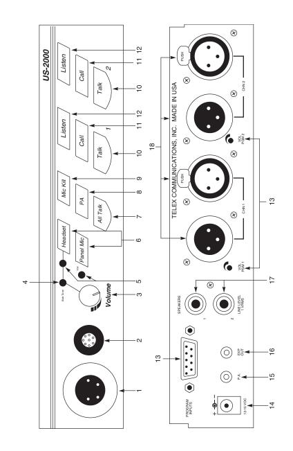
Figure 1. Front and Rear Panel Controls
