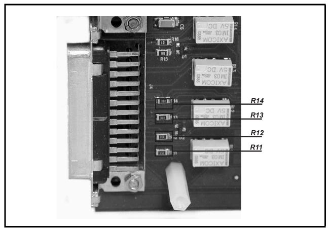
FIGURE 7. Cronus board resistor placement (9030-7788-001)
