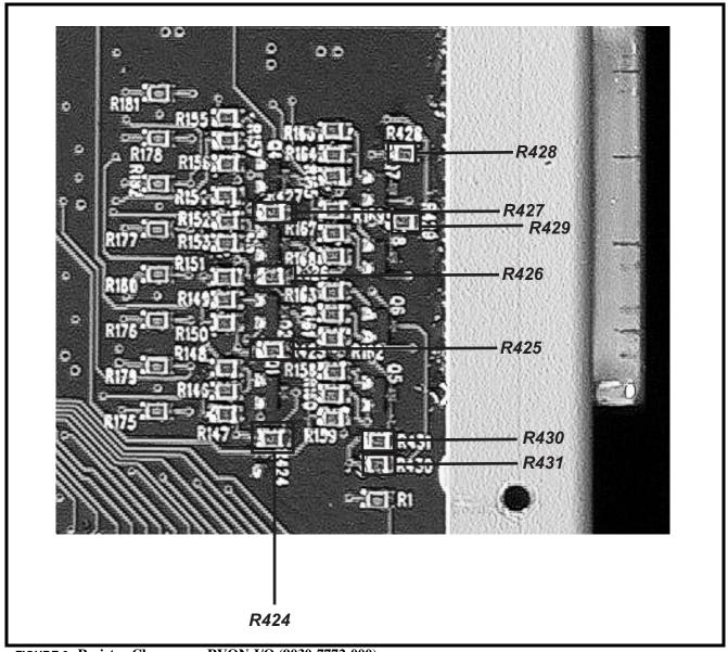
FIGURE 6. Resistor Changes on RVON-I/O (9030-7772-000)
