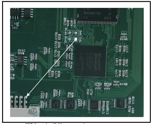
FIGURE 3. TP7 Ground to J3 C1 connector placement
