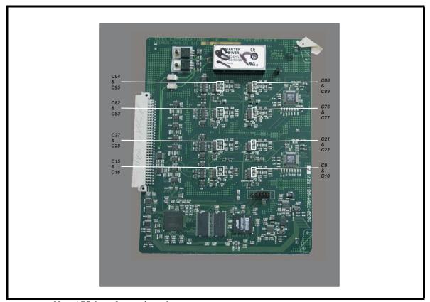
FIGURE 4. New AIO board capacitor placement
