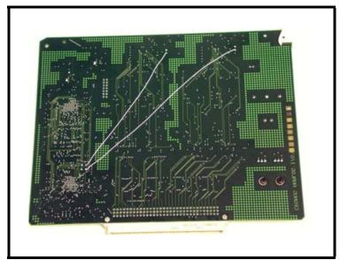
FIGURE 1. Wire Placement on the Cronus Front Card
