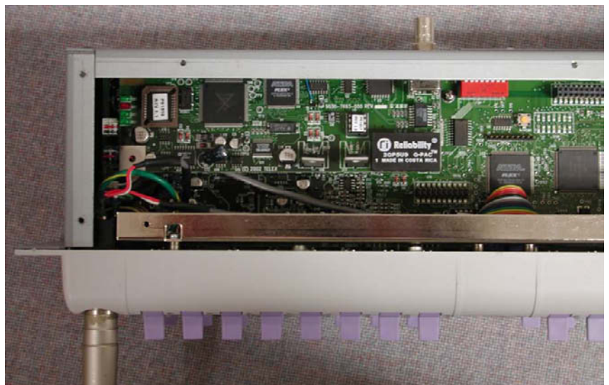
Figure 6 - View of installed CSI-100 board.
