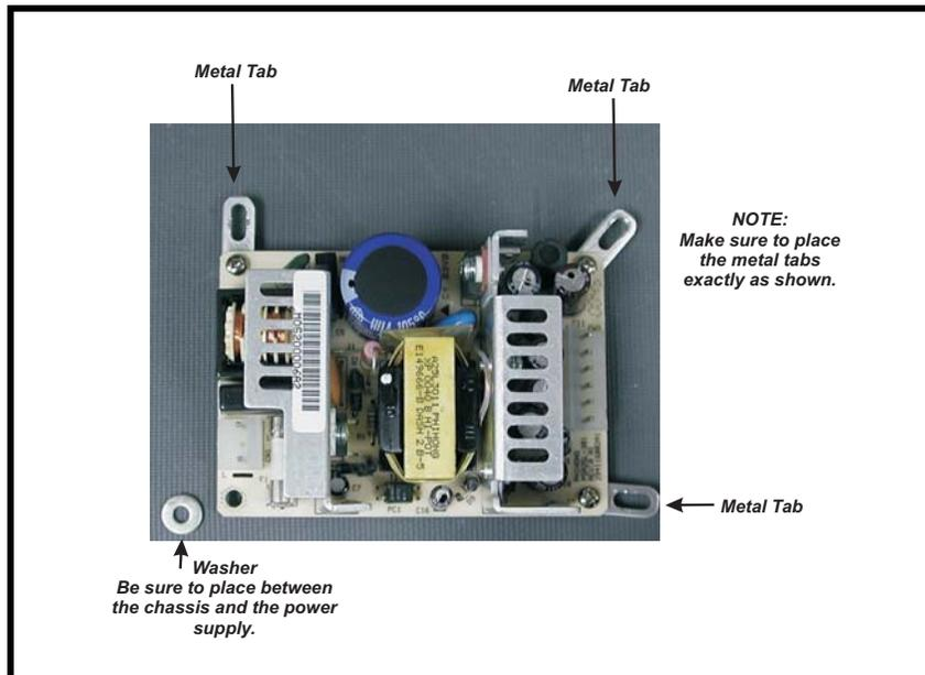
5. Using the screws from the old power supply, attach the power supply to the chassis.
