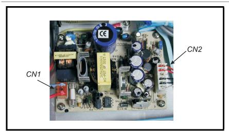
**3.** Remove the **four (4) placement screws** and remove the power supply. *Set the four screws aside, they will be used to remount the new power supply.*
