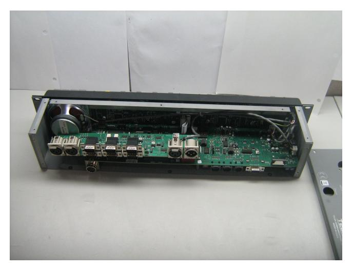
3. Continue disassembly process and remove the Noritake display boards from the front panel.
