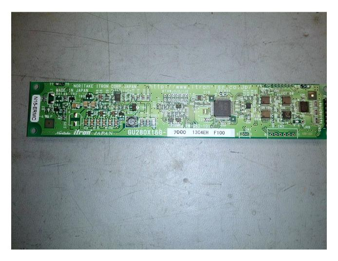
Note the part number GU280X16G-7000 marked on the display PCBA and on the lower left side of the board notice the pads for capacitor C35.
