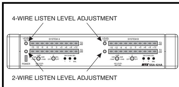
**FIGURE 8.** Location of level adjust trimmers
