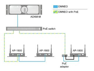
Figure 5. Connecting a single PoE-enabled AP-1800
