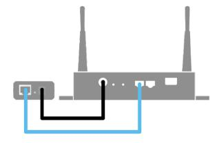
Figure 3. How to connect the PoE adapter
