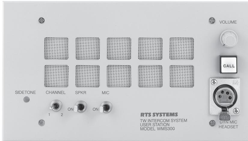
The WMS-300L Wall Mount Speaker Station is part of a series of user stations especially designed to work within the TW (Two-Wire) Intercom System. It fits directly into a standard 4-gang electrical conduit box (2.25 inch deep). The rear section is not enclosed and uses the back-box to provide a housing when installed.
