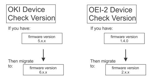
The following migration path determines the firmware files required for the KP Series panels.
