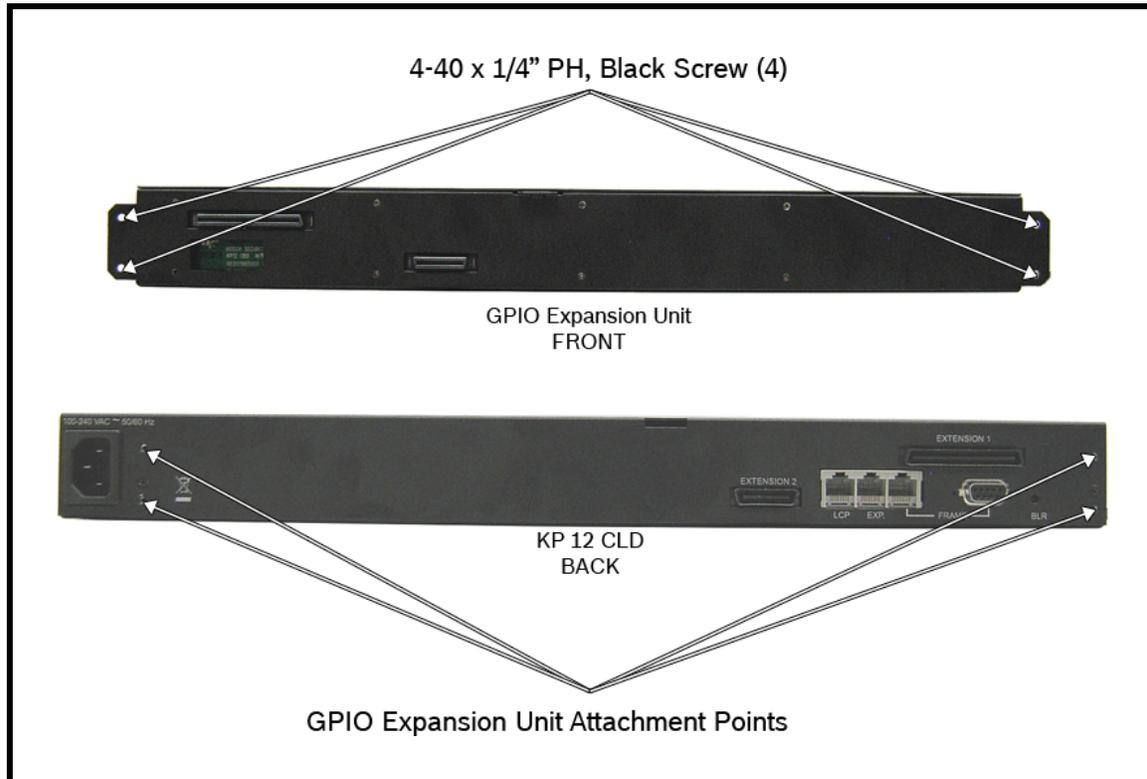
**FIGURE 2.** GPIO Expansion Unit — Attachment Points
