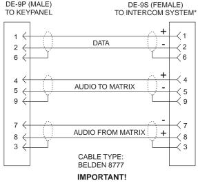
\* When connecting to an ADAM CS back panel, use only low-profile cable connectors such as AMP Part No. 747516-3 (Telex Part No. 59926-678)
