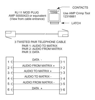
Figure 2. RJ-11 Intercom cable wiring diagram
