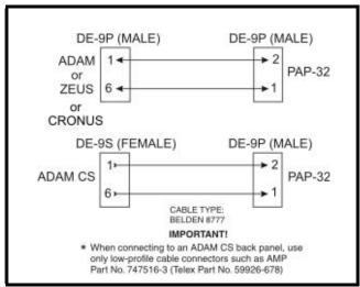
FIGURE 3. PAP-32 D-Sub Cable Diagram
