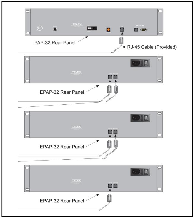
FIGURE 6. PAP and EPAP connection diagram
