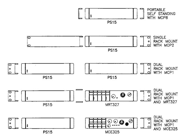
Installation Illustration—MCP Components
