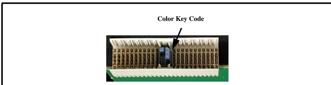
**FIGURE 1.** RVON-8 Color Key Code. This Key Code only allows the RVON-8 to plug into an RVON8 compatible backcard.
