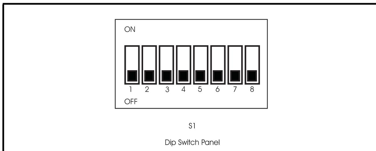
**FIGURE 2.** RVON-8 Dip Switch Panel
