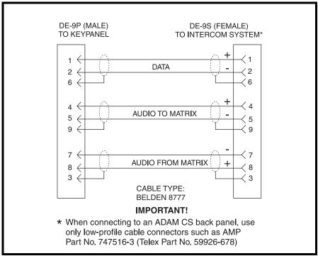
FIGURE 7. DE-9 Intercom Cable Wiring Diagram
