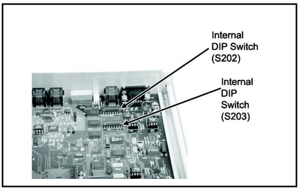
FIGURE 3. TIF 2000 Internal DIP Switch Locations
