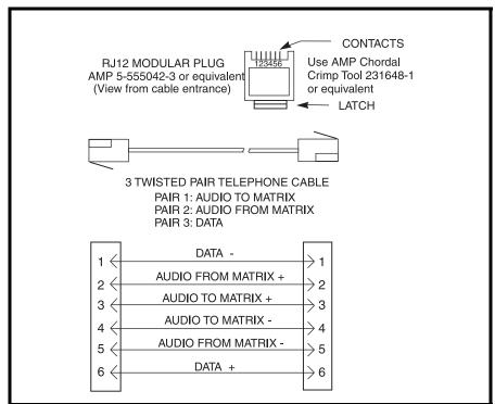
FIGURE 6. RJ-12 Intercom Cable Wiring Diagram
