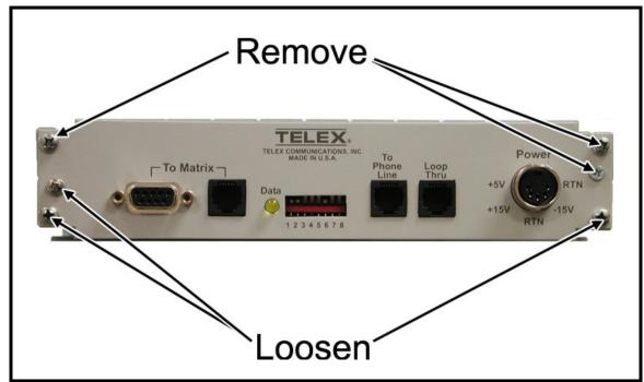
FIGURE 4. TIF 2000 Chassis Screws
