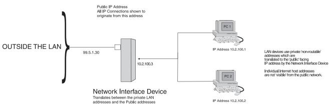
Note: A Network Interface Device can be a router, switch, gateway or anything that acts as one of these devices, such as a PC.
