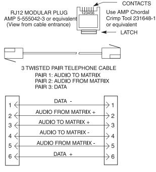
FIGURE 2. RJ12 Intercom Cable Wiring
