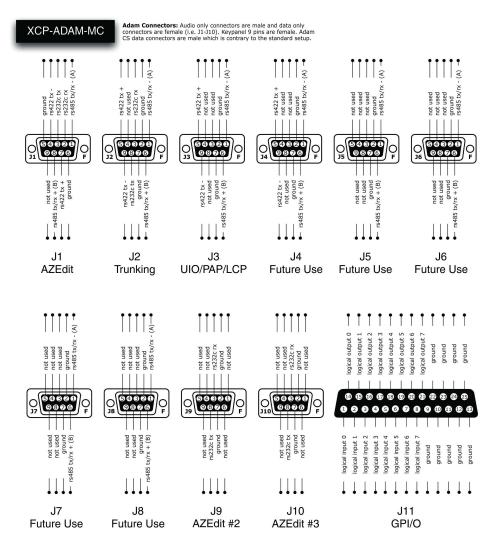
**NOTE:** AZedit sessions are only enabled on J9 or J10 when the advanced communication boxes are enabled from "communications" screen and the correct baud rates are configured.
