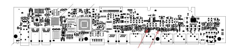
Close-up View of resistor locations R403 and R602:
