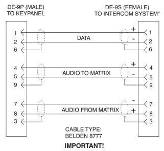
\* When connecting to an ADAM CS back panel, use only low-profile cable connectors such as AMP Part No. 747516-3 (Telex Part No. 59926-678)
