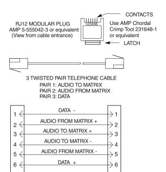
Figure 5. RJ-11 Intercom cable wiring diagram
