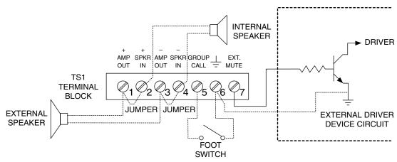
Figure 7. Terminal block wiring diagram for KP-96-RC option
