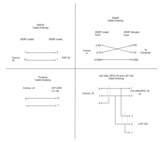
FIGURE 31. Cable drawings for PAP-32, AZedit, Trunking and UIO-256/GPIO-16/LCP-102
