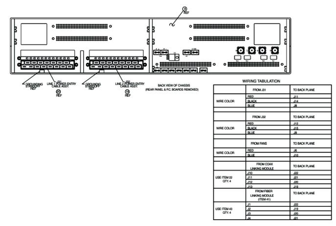
FIGURE 11. Wiring Diagram for Cronus
