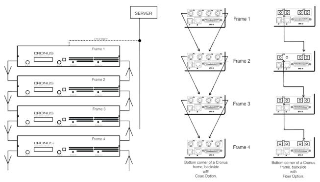
FIGURE 5. System Diagram and Frame Cabling
