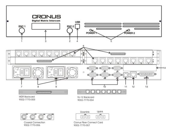
FIGURE 1. Controls, Connections, and Cronus backcard.
