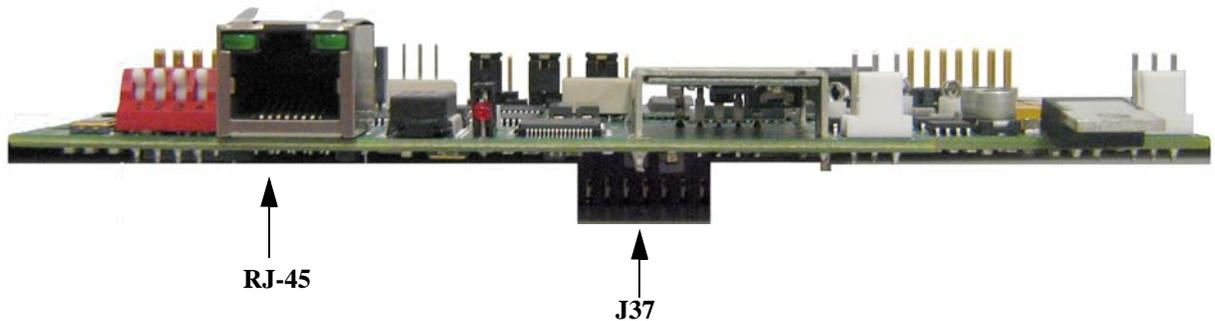
3. Connect the **RJ-45 extension connector cable** to the RVON-1 board.
