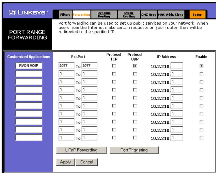
**Figure 7.** Router Configuration Window
