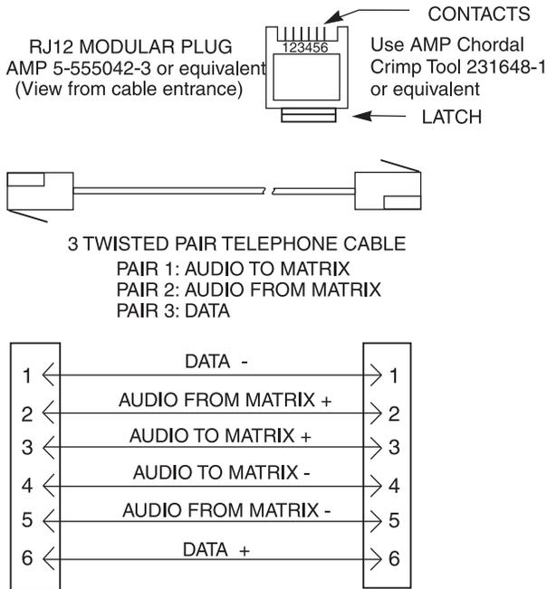
FIGURE 2. RJ12 Intercom Cable Wiring
