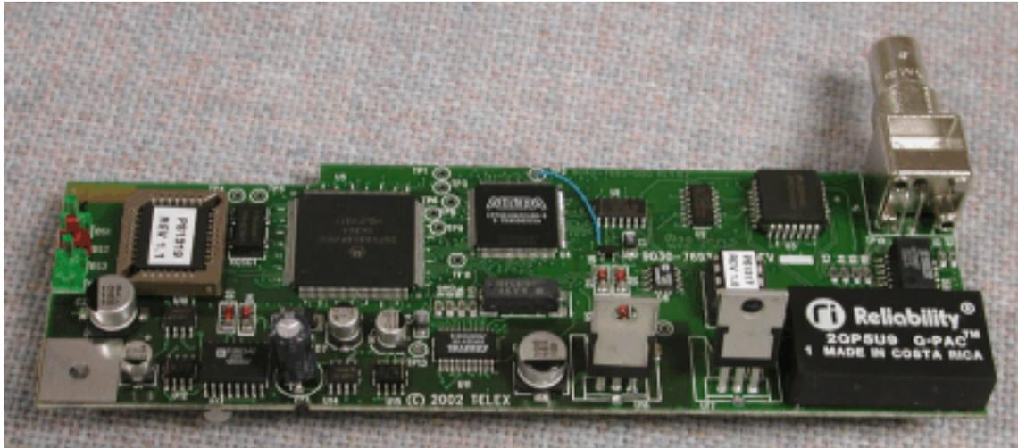
FIGURE 3. KP-632 CSI-100 coaxial system interface board.
