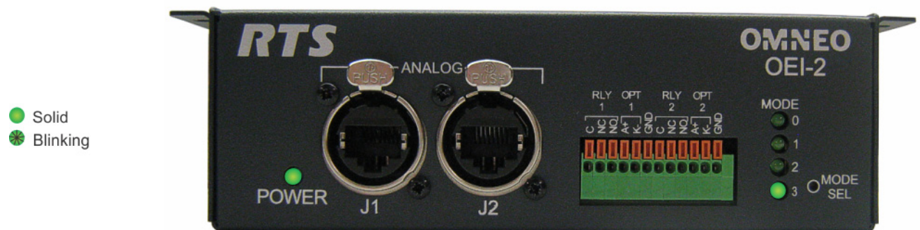
FIGURE 15. Single Keypanel – Channel 2 (LED 3 is solid)
