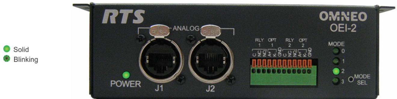
FIGURE 14. Single Keypanel – Channel 1 (LED 2 is solid)
