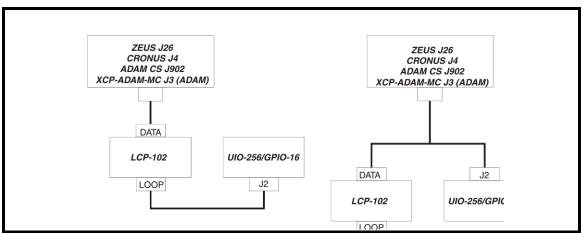
FIGURE 3. Connection example of an LCP-102 connecting to a UIO-256/GPIO-16
