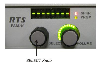
FIGURE 1. SELECT knob on the PAM-16 front panel
