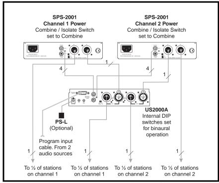
**FIGURE 8.** Using two SPS-2001 Power Supplies to provide a greater capacity on each channel. Using two SPS-2001 Power Supplies also lets you independently monitor and adjust volume for both intercom channels without the need for a separate powered loudspeaker. In this application, the US-2000A should be set for binaural speaker output as described in the US2000A manual.
