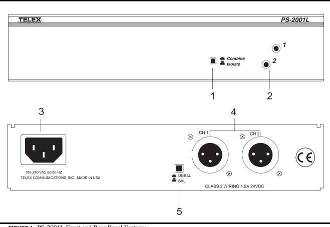
FIGURE 1. PS-2001L Front and Rear Panel Features
