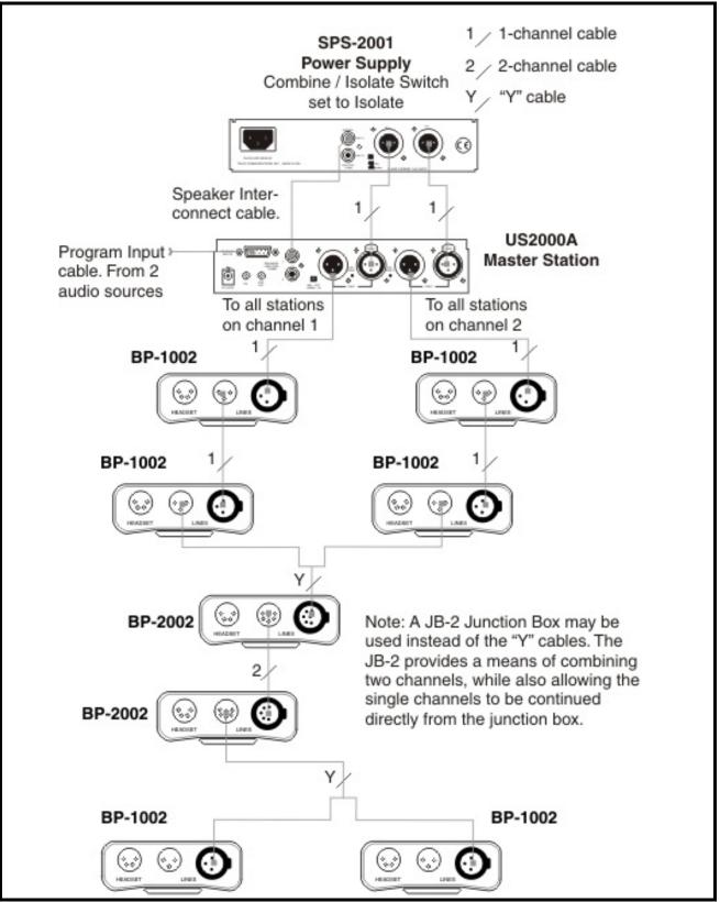
**FIGURE 5.** Typical connections using on SPS-2001 Power Supply for two intercom channels. The two program sources are monitored independently by their intercom channels. All audio (program and intercom) is monitored as a monaural mix in the SPS-2001 speaker. The US2000A is set for monaural speaker output (default).
