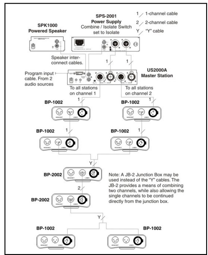
**FIGURE 6.** The two program sources are monitored independently by the intercom channels. The SPS-2001 monitors intercom channel 1 and program 1. The SPK-1000 monitors intercom channel 2 and program 2. The US2000A is sent for binaural speaker output as described in the US2000A User Manual.
