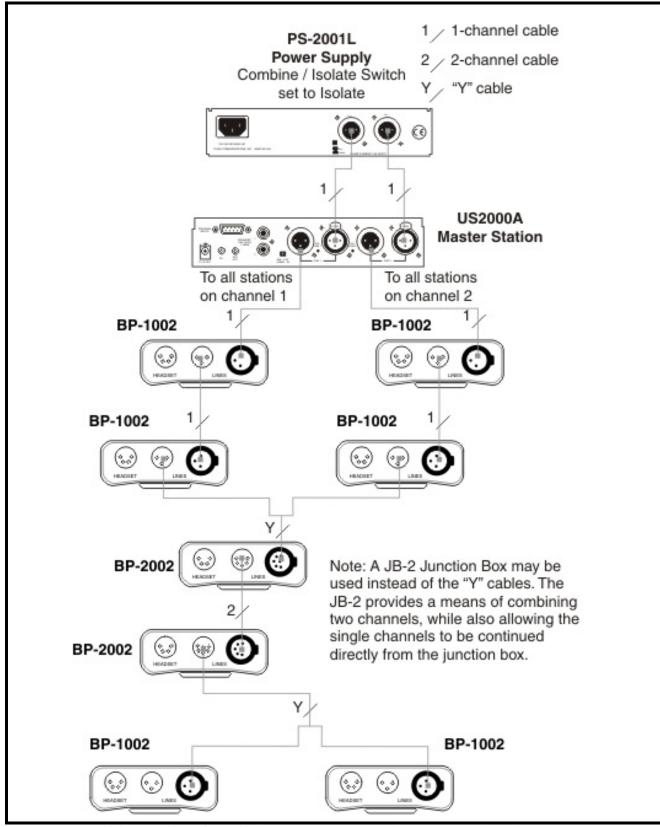
FIGURE 4. Typical connections using a single PS-2001L Power Supply to power two channels.
