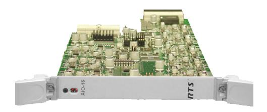
Installed directly into the ADAM or ADAM-M Matrix Intercom System, the AIO-16 card gives 16 ports of audio in and out for each card installed. This doubles the amount of audio ports available from its predecessor the AIO-8. The AIO-16 is hot swappable, allowing the user to insert the card and begin using it instantaneously. Once inserted into the system, it uses its "smart card" capability to see the backcard configuration and switches its keypanel communication protocol accordingly.
