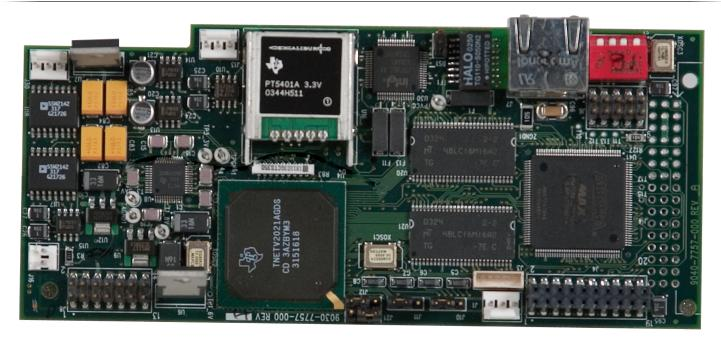
Installed directly into KP-32 or KP-812 keypanels, the RVON-1 provides **VoIP** (Voice over Internet Protocol) communications for the RTS ADAM intercom family. VoIP means sending voice information in digital form using discrete packets rather than the traditional hardwire connection. The RVON-1 delivers an integrated solution for connecting keypanels to the intercom matrix over standard IP networks.
