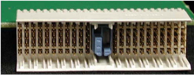
FIGURE 3. The RVON-16 Color Key Code. This Key Code allows only the RVON-8 or RVON-16 to plug into a blue coded, compatible backcard.
