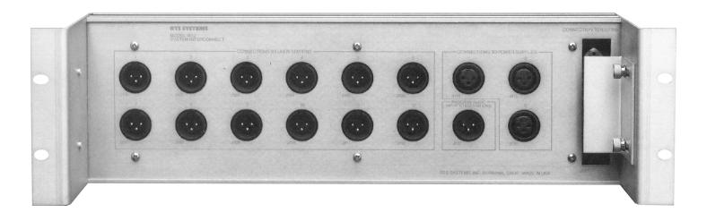
The RTS Model 4012 System Interconnect is a 19 inch, 3 **RU** (Rack Unit) system interconnect. It has a 50-pin to 3-pin XLR connector transition assembly. The 4012 is used with the 800 Series Master Stations. The 4012 translates the 50-pin connectors to 12, 3-pin XLR male connectors. Additional connectors are provided to apply power to XLR connectors.
