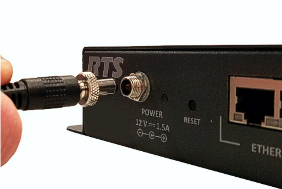
2. Plug the **power cord** into the device.
