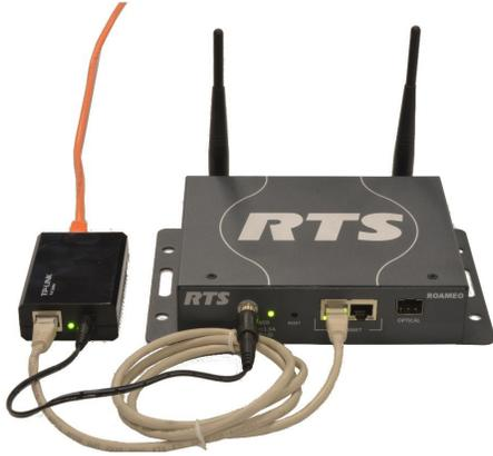
Figure 3. How to connect the PoE adapter
