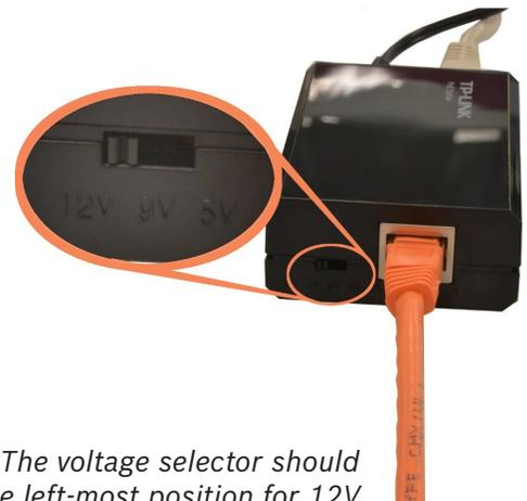
Figure 2. The voltage selector should be in the left-most position for 12V
